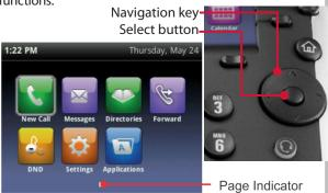
To get to different icons, you can use the right, left, up, and down arrow keys on the **Navigation** key (shown above right). To choose an icon, press the **Select** button in the center of the **Navigation** key.
